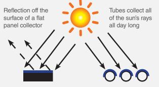
Evacuated tubes catch and keep the sun's radiation, and reflects less of the sun's energy.
