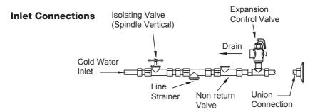
**Note:** a combined isolating valve/non-return valve/line strainer may be used. Expansion control valve only required where local regulations demand.
