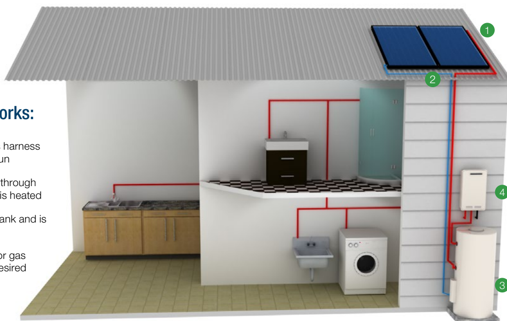
Illustration of gas boosted SplitLine system
