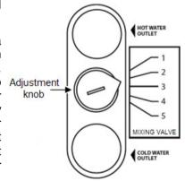
Adjusting the mixing valve adjustment knob to position '5' will allow water to be delivered at the stored temperature of the cylinder (no mixing). Each numbered incremental change from position '5' represents a temperature decrease of approximately 5°C (incremental increase of cold water mixing).
