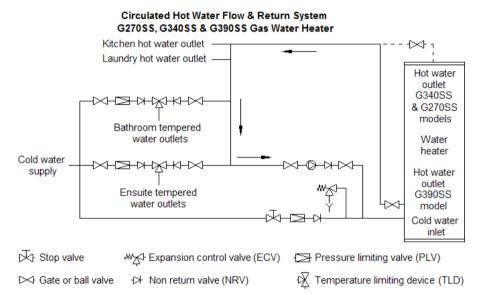
**Note:** NRV's shown on cold & hot water supply lines to TLD's are required if not incorporated in TLD
